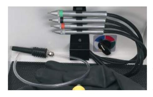
**BASE EVO** working chamber showing the recycling projector (yellow, below), four microprojectors fixed in their practical holder and the rubber air blower.
