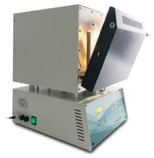
Burn-out furnace with simplified electronics. Two distinct working cycles. The first program has been developed specifically for quick investments, featuring a fast rise in temperature, time control stabilization and warning at the end of the cycle (repeat function). The second program is most suitable for traditional investments and can offer up to three temperature thresholds with adjustable rising gradients and holding times which can be preset according to specific requirements.
