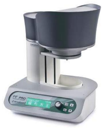
Inside the firing chamber, a quartz filter allows to boost the effects of IR rays, thus ensuring progressive heating of the firing objects whilst controlling evaporation of humidity. The temperature is detected by a special, oxidation-free thermocouple which does not require periodical adjustment
