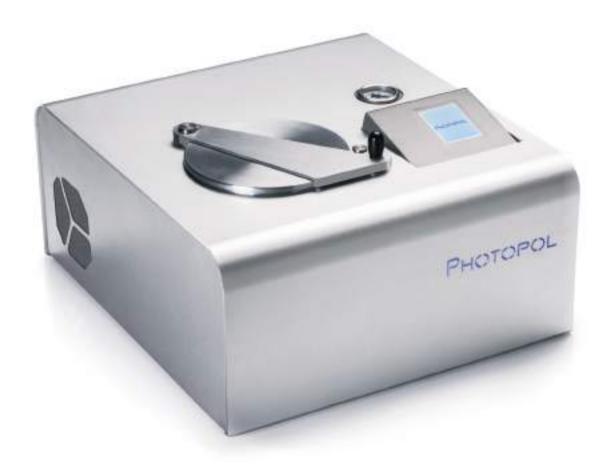
PHOTOPOL "VACUUM+GAS" (A5408V) is equipped with 6 special circuits (8-LEDs Hi-Power SMD, 48 LEDs in total) with optical reflectors, developed to maximize the irradiation effect. Thanks to its wide operating spectrum it allows to post-cure components created with 3D printers working both at a wavelenghts of 385nm or at 405nm.
