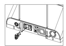
Reinsert the compartment in its place pressing firmly into the middle part of the fuse box.
